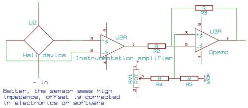
This is just an example of an offset voltage correction that gives good results. There are many other ways to compensate for offset voltages. As the electronics already has a current source, it is good practice to use the reference used for that current also as reference for compensation of offset voltages. This will cancel out part of the temperature drift of your electronics.
