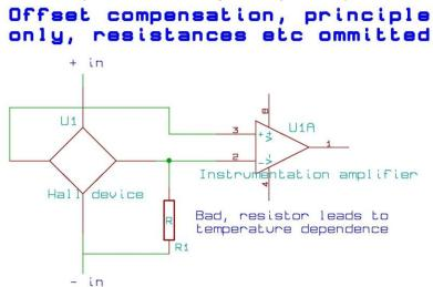
The example above leads to a temperature drift of the offset voltage. Meaning that the offset voltage is not constant but changes with temperature and is difficult to compensate. + in
